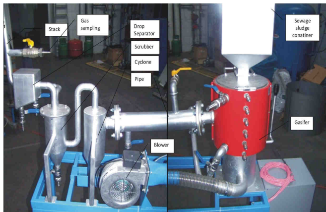
Fig. 4. Photo of the fixed bed gasifier installation
