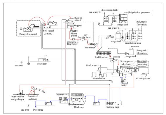
Figure 6. Flow of operation steps.
