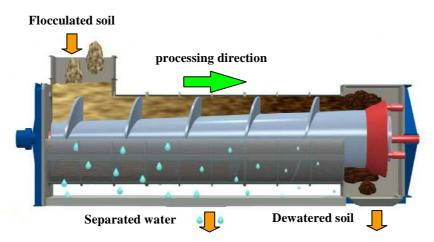
Figure 1. The principles of Eco-screw.
