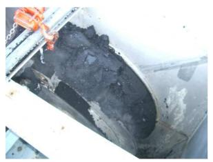
Photograph 10. Discharging dewatered sediment through outlet.
