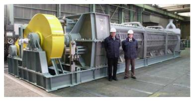
Photograph 1. Screw press of 1,350-mm diameter.
