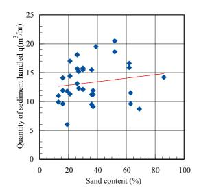
Figure 7. Sand content and quantity of sediment handled.
