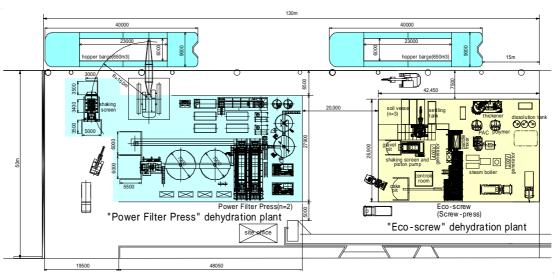
Figure 4. Plan of intermediate processing plant.
