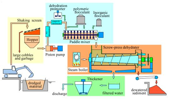
Figure 2. Standard operation steps for the Eco-Screw system.
