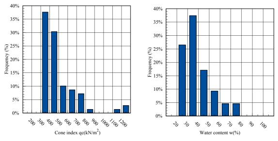
Figure 8. Mechanical properties of dewatered sediment.
