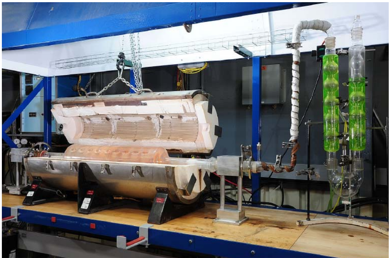
Figure Two: Batch Kiln System
