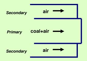
Mass flow fuel  $\rightarrow$  fixed Primary flow rate  $\rightarrow$  fixed Mass flow  $O_2 \rightarrow$  fixed  $O_2$  concentration func. of RFG second High  $O_2$  conc.  $\rightarrow$  less Secondary flow
