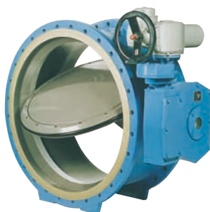
Keystone Dubex - RMI AWWA Butterfly Valves – Torque seated: greater torque results in improved tightness. Closing torque is in direct relation with the shutoff pressure, which results in smaller actuator selections at lower pressures. The resilient disc seal is replaceable in-line.
