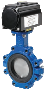
Keystone Figure 990/920 – One piece thin profile disc/stem allows for molding of elastomer or polymer and is also available in stainless steel or alloy materials. Thin profile allows for high C_v and good control.
