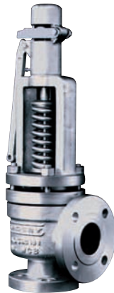
Crosby HL - Replaceable full nozzle with FLEXI-DISC® design; external blowdown bias adjustment for easier reseal setting.
