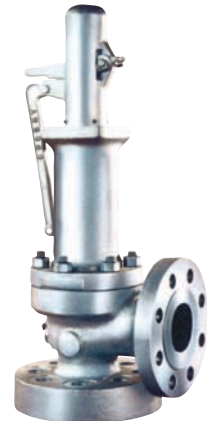
Crosby HSJ - Replaceable full nozzle with FLEXI-DISC® design; open or closed bonnet selection; for application in low pressure steam generators.
