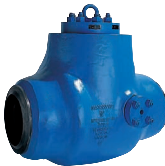
Intervolve Tilting Disc - Equipped with a dome to balance weight, and a spring-assisted closure to avoid slamming.
