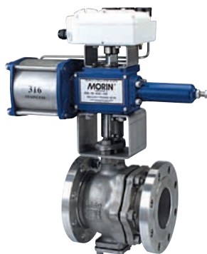
KTM Single V - Rotary-valve design provides shearing action between the V-notch ball and the seat, promoting a smooth, non-clogging operation.
