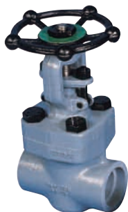
Hancock 950 - An unobstructed flow passage and metal-to-metal seating makes this valve ideal for applications where high velocity or highly viscous fluids must be handled with minimum flow loss.
