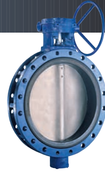
Keystone Figure 106 – Large diameter double flanged valve offered in a variety of seat and disc materials to meet many service conditions. Fully rubber lined valves are available for abrasive services.
