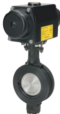
Keystone K-LOK – ASME Class 150 and 300 rated valves available with a soft seat, metal seat, or API 607 4th edition certified firesafe seat. Double offset design allows for high cycle life and less seat wear.
