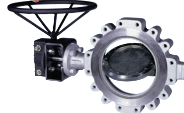
Vanessa QTL - Quarter-turn, non-rubbing design with a unique, triple offset geometry that eliminates all seat-to-seat rubbing throughout the valve's 90° rotation.
