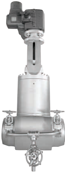
Raimondi Raisteam Valve - Forged body position seated isolation valves for severe service and critical isolation applications. Zero leakage seating design eliminates thermal binding.
