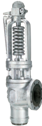
Crosby HCA-118W - Supercritical safety valve for start-up flash tanks, convection pass mix header, superheater and reheater for service to 5,000 psig [345 barg].
