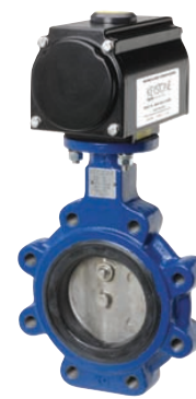
Keystone Figure 221/222 – Molded-in seat allows for 250 psi tight shutoff and lug style is rated for bi-directional dead end service at full pressure.
