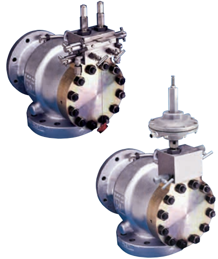
Anderson Greenwood 727 - High temperature metal trim design with advanced reverse flow technology; dual pilots with safety selector valve manifold available; optional as remote actuated dump valve.
