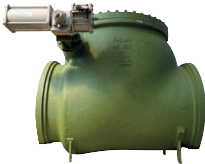
Fasani Steam Non-return, Power Assist, Positive Closure Check Valve - Designed to provide fast action closing before backflow and protect the steam turbine against reverse flow. Designed to B16.34 in sizes 6" through 60" and available with counterweights on sizes 10" and larger, if required.
