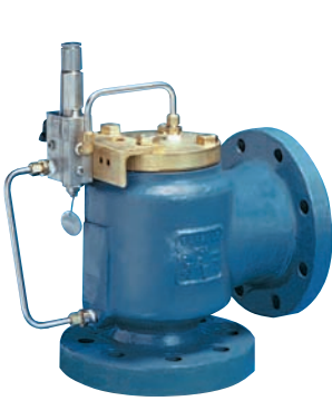
Anderson Greenwood 200 Series - Balanced design of pilot operated valves ensures that proper valve operation and lift are unaffected by back pressure. Costly and fragile metal bellows are not required.
