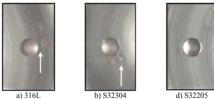
Figure 9: pictures of coupon surfaces after the immersion test in 50g/L NaCl solution at pH 6.4 and 50°C (white arrows indicate crevice attacks).
