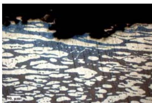
Figure 10: picture of a UNS S32304 cross section sample in the crevice corroded area under the MCA after 1000h immersion in 50g/L NaCl solution at pH 6.4 and 50°C (NaOH etching).
