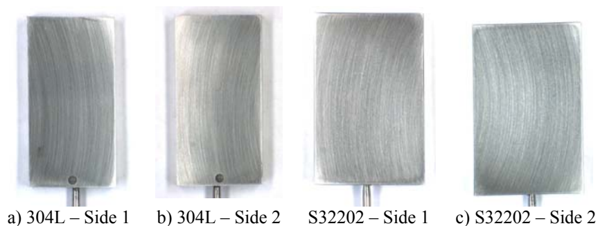
Figure 21: pictures of surfaces after the immersion test in 1000ppm chloride ion solution at pH 4.5 and 25°C.
