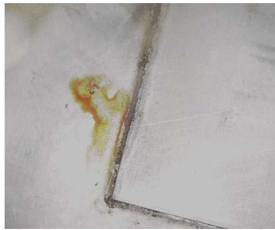
Figure 12: photograph of pitting attack on 316L, shown by arrow on Figure 11
