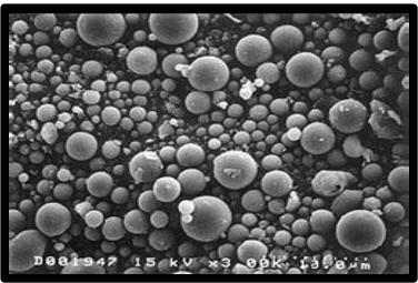
Electron Microscope (SEM): Fly ash particles (Cenospheres) at 2,000 x magnification, from FHWA DOT Gov.jpg
