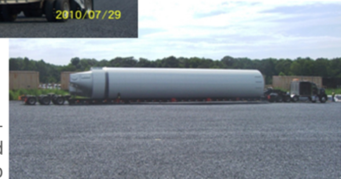
Shop-fabricated Lime Day Silo
