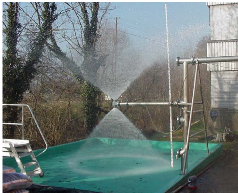
Figure 10: Bi-directional spray nozzle testing
