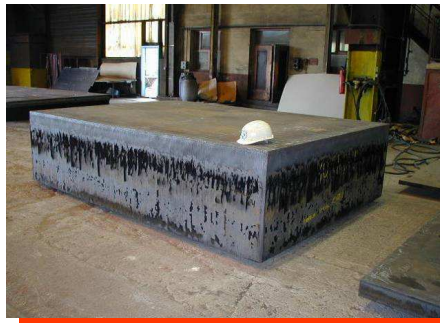
Pre-hardened thick block up to 37.4" thick (950 mm)
