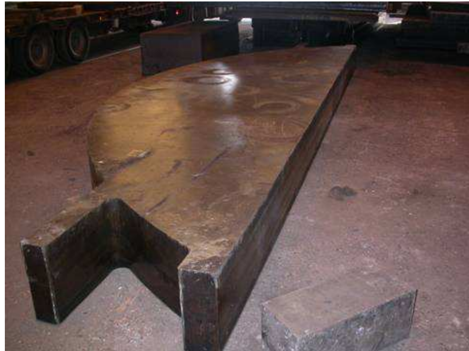
17.7" thick ¼ tube sheet (>315" diameter) Oil and gas applications
