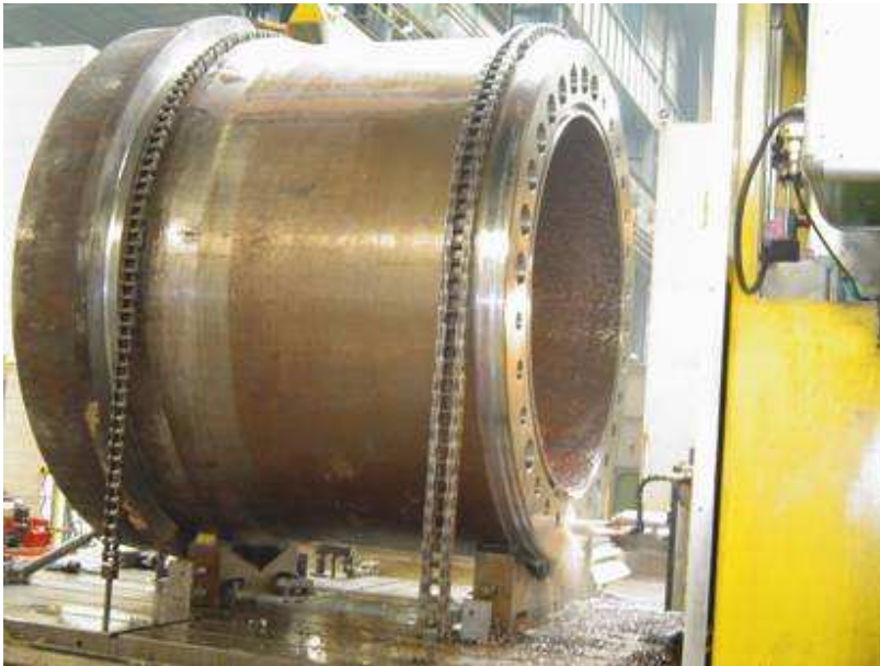
Cylindrical part of the jack (AISI 4142)
