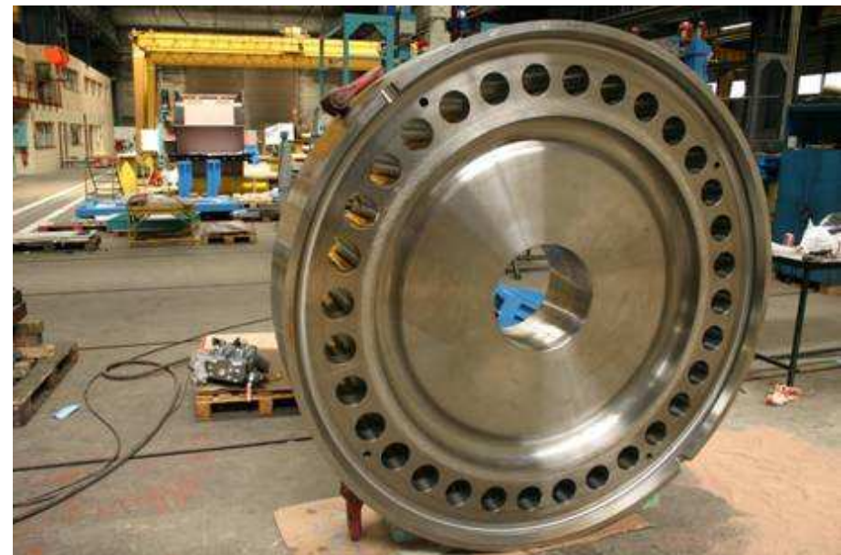
New head made from a 28.3" thick Mecasteel 75 block
