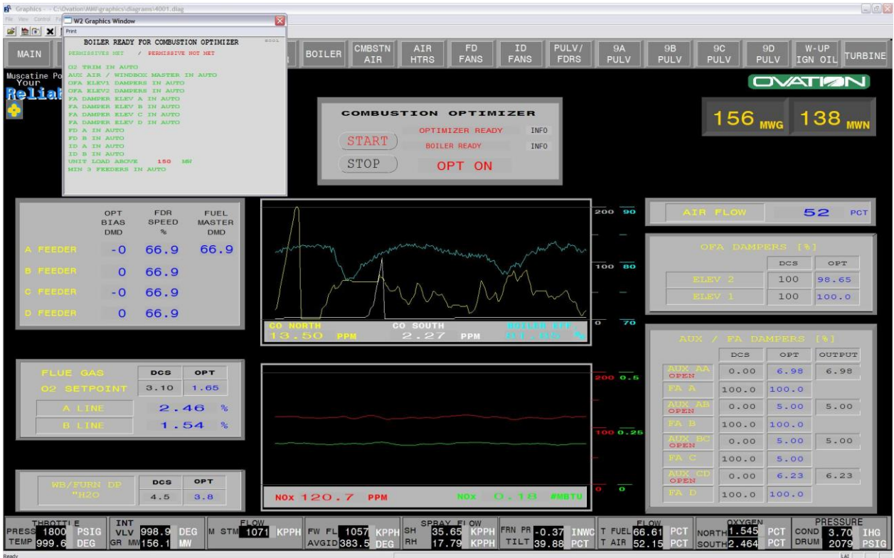
Figure # 9 Boiler Ready Signals for Combustion Optimizer
