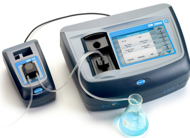
Figure 2: Sipper cell for improved sensitivity
