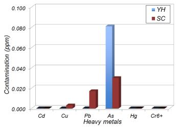
FIGURE 3: The graphs of degree of contamination by leaching test
