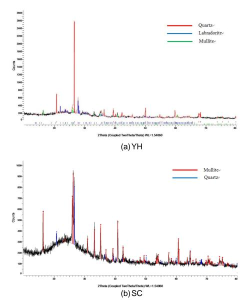
FIGURE 4: Results of the XRD analysis for YH and SC sample
