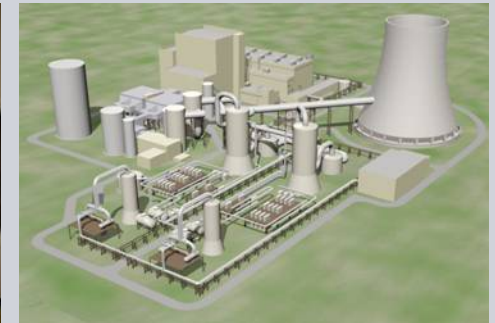
Post-Combustion Carbon Capture Plant Design
