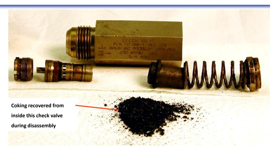
A standard Liquid Fuel Check Valve showing the realized coking potential.
