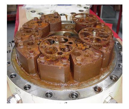
New flow divider design using exotic metals to prevent corrosion. Does not resolve fuel evacuation.
