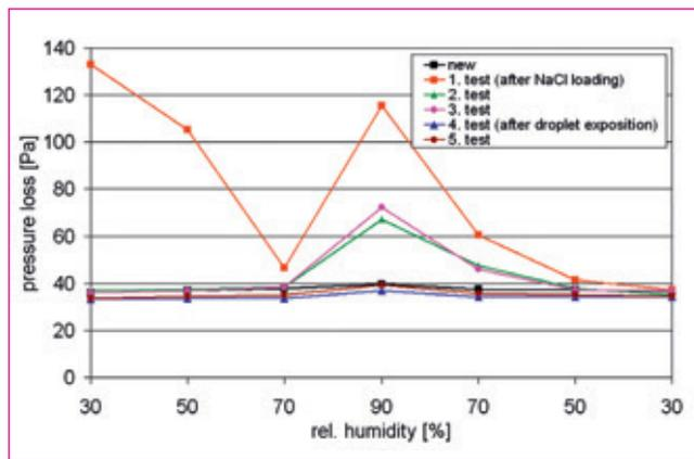
Fig. 8: Media test with water droplets
