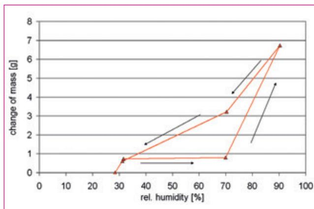
Fig. 4: Media test (filter surface area: 600 mm x 300 mm, volume flow: 80 m<sup>3</sup>/h, T: 23°C)
