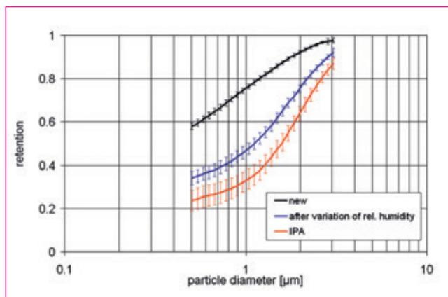
Fig. 10: Fractional separation efficiencies of the tested filter media (DEHS test aerosol)
