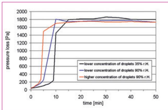
Fig. 7: Media test with water droplets (volume flow: 80 m<sup>3</sup>/h, T: 23°C, filter surface area: 600 mm x 300 mm)
