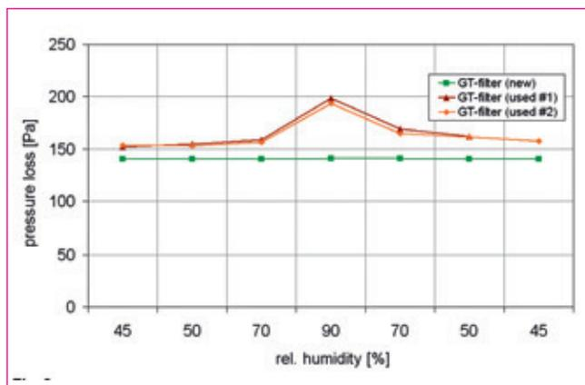
Fig. 9: Pressure loss measurements of used gas turbine filters (carried out on the HVAC test bench according to DIN EN779-2012 [5] and provided by the Institute for Energy and Environmental Technology, Duisburg
