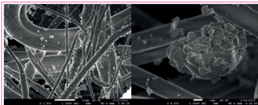
Fig. 6: Media test + NaCl/A2 exposure without/with moisture variation
