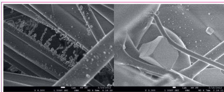
Fig. 5: Media test + NaCl exposure without/with moisture variation
