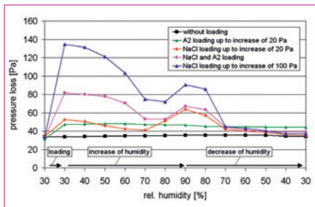
Fig. 3: Media test (filter surface area: 600 mm x 300 mm, volume flow: 80 m<sup>3</sup>/h, T: 23°C)
