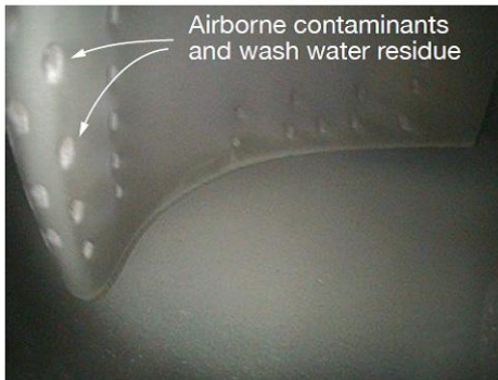
1. Airborne contaminants and wash water residue plug cooling holes in a first-stage HPT blade. Engine was not equipped with HEPA filters
