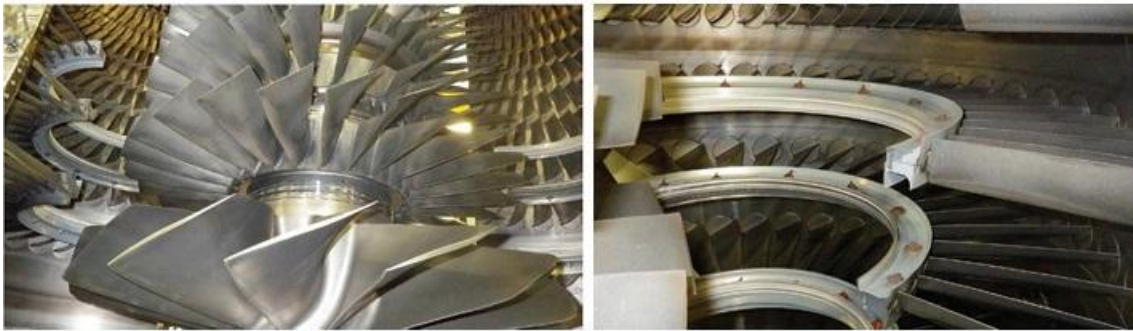
5, 6. Windfall Unit 1 compressor looks new after having operated for 31 months (more than 22,000 hours) at base load with no water washes
