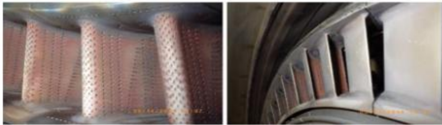
1. LM2500 first-stage nozzles have operated for 43,000 hours; the last 18,000 hours the engine was protected by hydrophobic HEPA filters. Cooling ports in the leading edge (left) are clear and there are no burn marks on the airfoils. Trailing edges at right are clean and exhibit no erosion, cracking, or platform deformation
