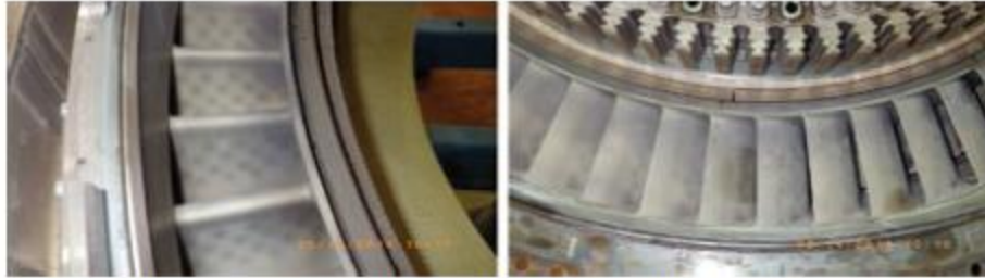
3. Second-stage nozzles look almost new—leading edges at left, trailing edges at right
