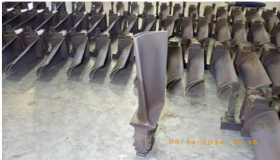
4. Looking at the tip and tip cap of this second-stage rotating blade you might think it new, certainly not an airfoil with 43,000 hours of service
