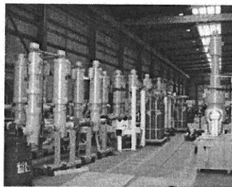
Slab gate valves are lined up and ready to go.
