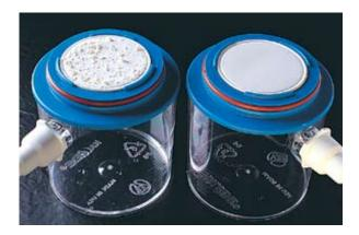
Spallation debris collected onto a microporous filter membrane after recirculating water for 48 hours through thermoplastic elastomer tubing (left) and GORE™ High-Resilience Tubing Style 100SC (right.) The thermoplastic elastomer tubing produced particles of rubber, inorganic filler and plasticizer. There was no shedding from the GORE™ High-Resilience Tubing Style 100SC.
