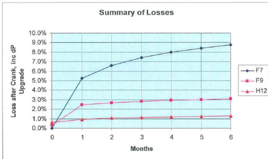
Figure 3-3. Comparison of Gas Turbine Degradation with Different Levels of Filtration (Owens, 2009)
