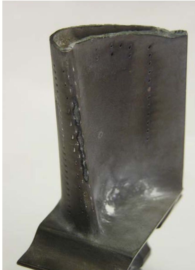
Figure 2-4. Erosion on the Leading Edge of a Turbine Blade
