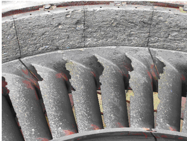
Figure 2-2. Gas Turbine Damage from FOD
