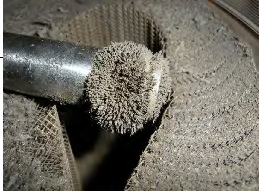
Magnetite debris from filter (magnetic)
