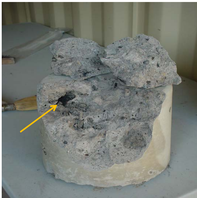
Figure 1 – Example of Solidified/Stabilized Material with Coal Tar Inclusion
