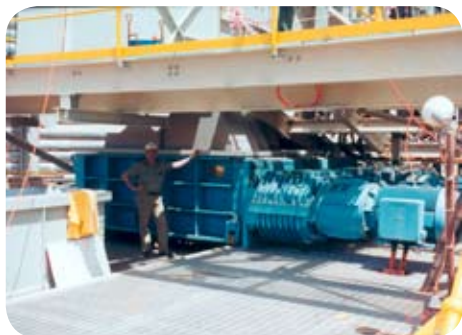
4400 t/h Primary ABON Sizer, crushing bauxite
