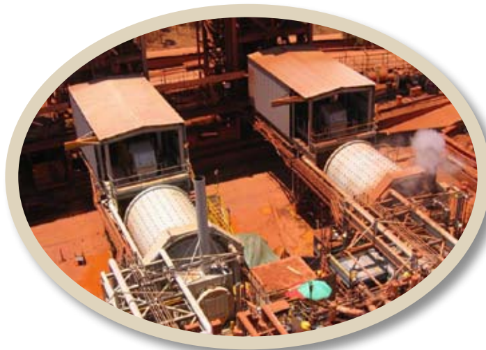
World's largest Rod Mills on Bauxite at Gove , Australia
