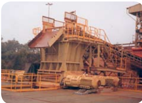
2500 t/h Secondary ABON Sizer, crushing bauxite
