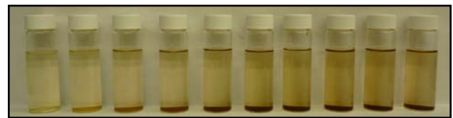
Fig. 5 Mn_xO_y -rich precipitate formation from spiking of filtrate from corroded unit into control filtrate.
