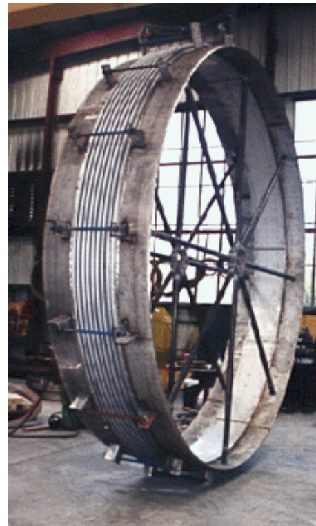
Typical internal spider for metal gas turbine exhaust joint
