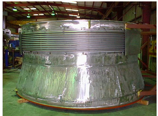
Completed Metal GTX Transition Assembly for Siemens Turbine V84.3A
