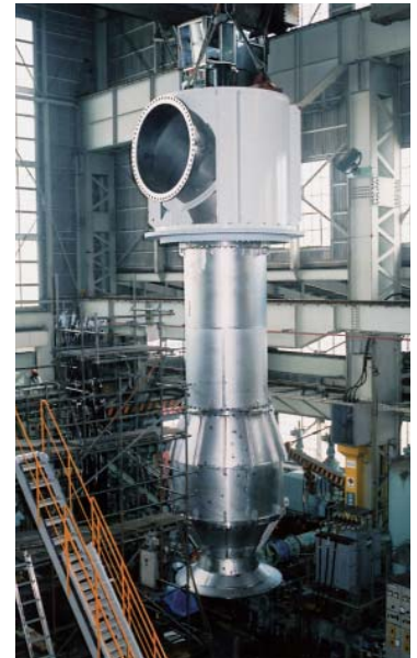
Circulating Water Pump
