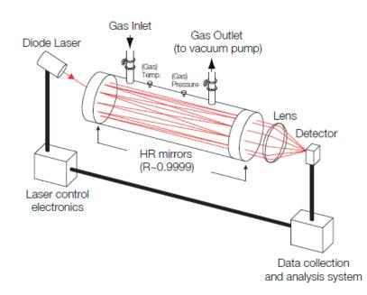
Setup for LGR's patented Off-Axis ICOS technique
