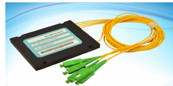
Figure A-12 4-channel Multiplexer
