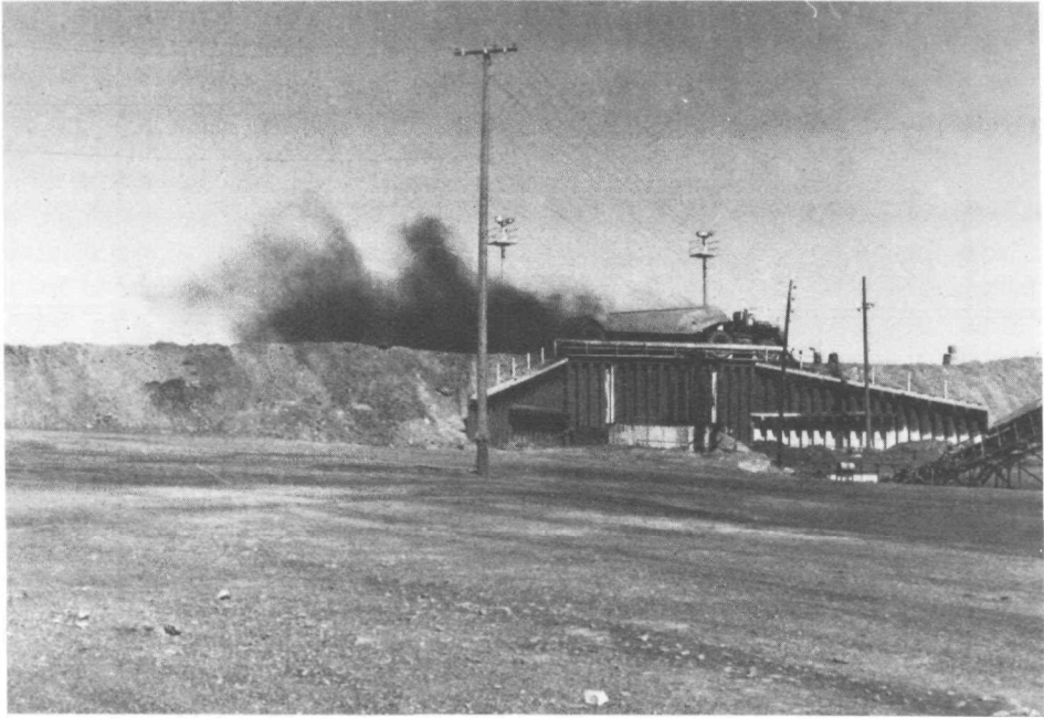
Figure 4-6. Example of fugitive dust from unloading at a coal mine.
