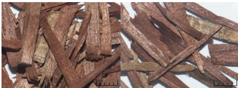
Before and After Grinding for 6 min in a 3" Ball Mill
