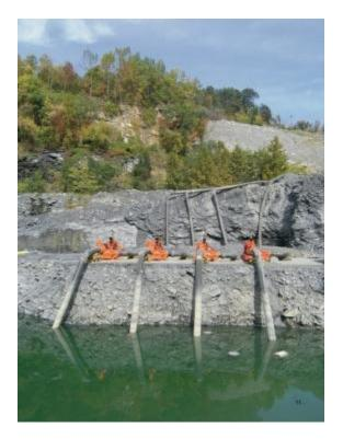
Godwin Pumps offers an unparalleled line of extreme high lift horizontal single-stage centrifugal pumps for the world's toughest mine and quarry dewatering assignments. Capable of heads to 650' using a single impeller up to 20" in diameter, just one Godwin extreme high head pump can provide the same pumping capacity as several of its multi-stage competitors.
