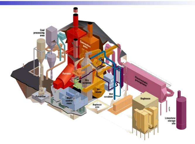
Operations focused on combustion, heat transfer and Air Quality Control Systems
