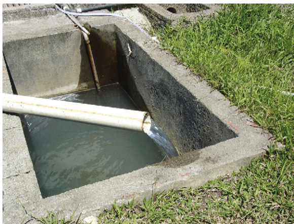
Fig. 13. Treated water in a FGR–FADAT pilot unit. Same AMD as in Fig. 12.
