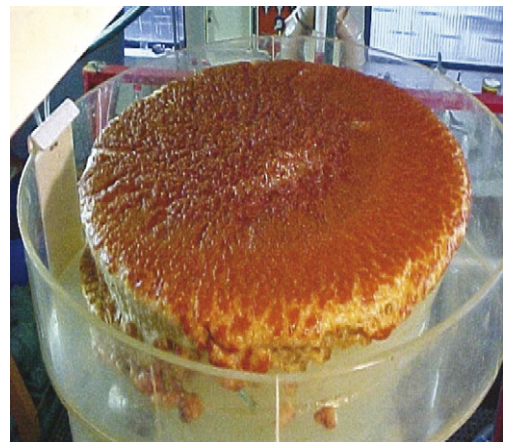
Fig. 4. Colloidal iron precipitates, \text{Fe}(\text{OH})_3 , floated by DAF, without collector.
