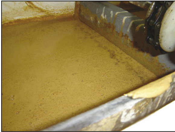
Fig. 12. Floated product in a FGR–FADAT pilot unit treating an Acid Mine Drainage (AMD) from a coal mining.
