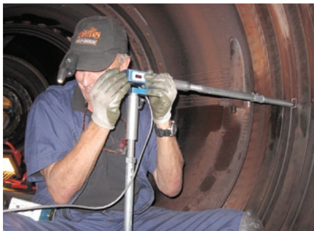
4-14. Actual casing centerline was needed to assure proper reassembly
