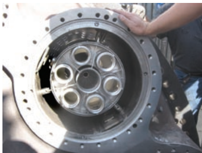
4-30. Liner inserted in flow sleeve
