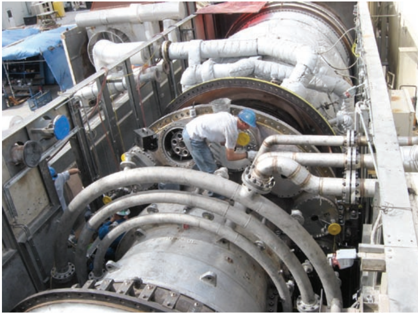
4-34. Fuel manifolds in foreground: Primary at top, transfer in middle, secondary at bottom
