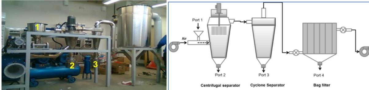
Figure 2 Photo and schematic diagram of the fly ash separation system at NICE
