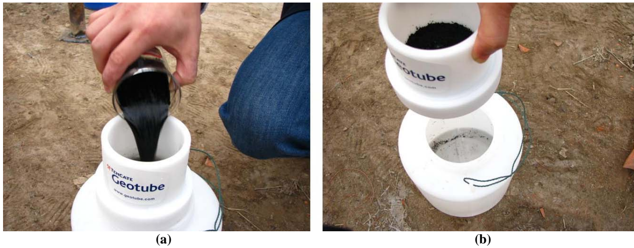
Figure 18. RDT performed at Tianjin Eco-City (a) pouring sample into funnel (b) visual observation of solids retention and clarity of effluent.
