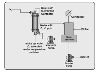
Membrane Contactors can be used to remove the dissolved oxygen from boiler water. With the proper configuration and system design Membrane Contactors can remove essentially all of the dissolved oxygen present in the water stream. Membrane Contactors can be used as stand alone Deoxygenation systems or they can be used with existing technology as a hybrid system.
