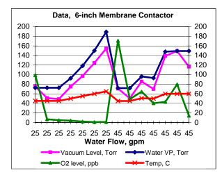
A review of the data shown in the graph indicates several very important points regarding the use of a membrane contactor for this application. An initial key point is that dissolved oxygen levels can be reduced to well below 10.0 ppb with a single contactor. In more "traditional" membrane contactor designs several contactors in series are typically required to reach these lower levels of dissolved oxygen.
