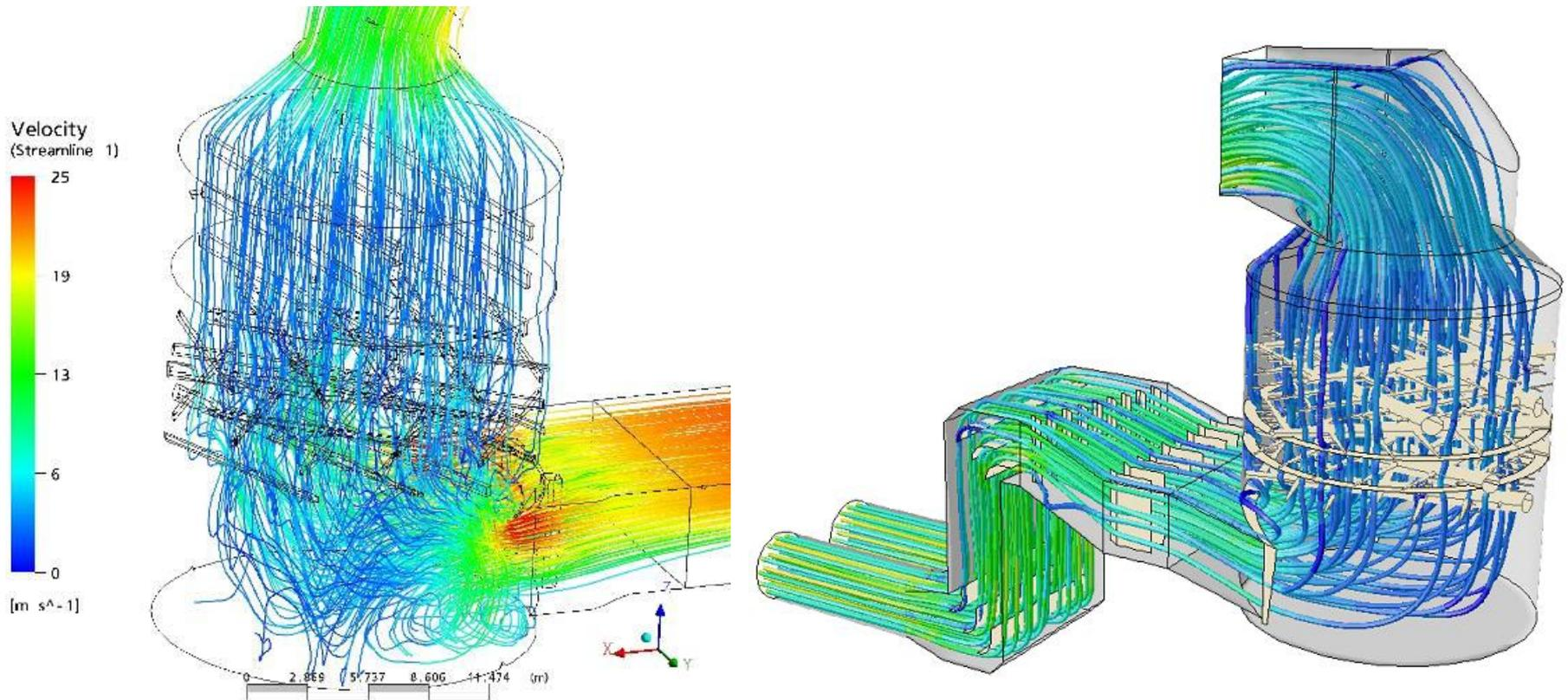
**Inlet duct design and spray pattern, spray nozzle placement and wall ring prevents channeling and distributes gas over the entire cross section while delivering even slurry spray.**
