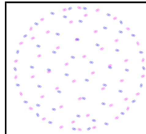
Adjacent levels are offset from one another to provide complete coverage, prevent channeling, and minimize wall sneakage.
