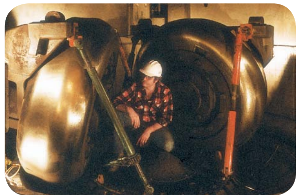
▲ A single, large access door, small footprint and specially designed tooling are features of the B&W Roll Wheel pulverizer that help reduce maintenance costs.
