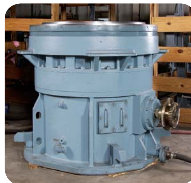
▲ The planetary geardrive is a compact option for select pulverizer installations.
