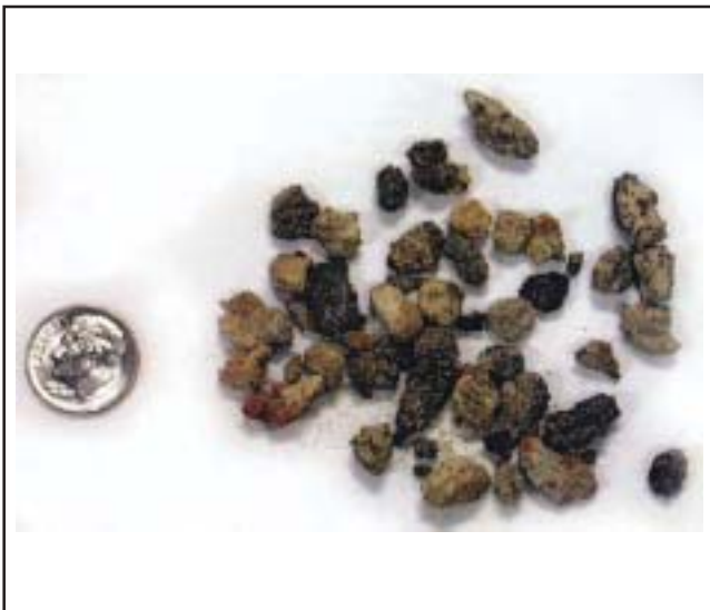
Fig. 9 Karn SCR units were designed to handle large particle (popcorn) ash, if it is ever encountered.
