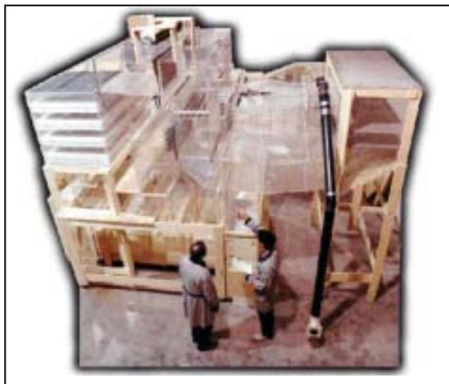
Fig. 6 Typical physical SCR model.
