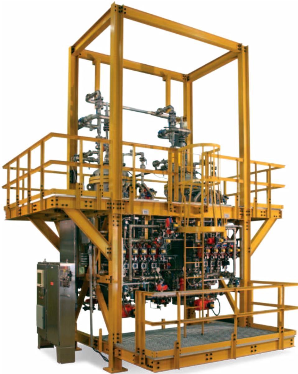
Duplex candle filter system in the fabrication shop consists of two candle filters, piping, wiring and complete PLC system with communication back to the refinery DCS.
