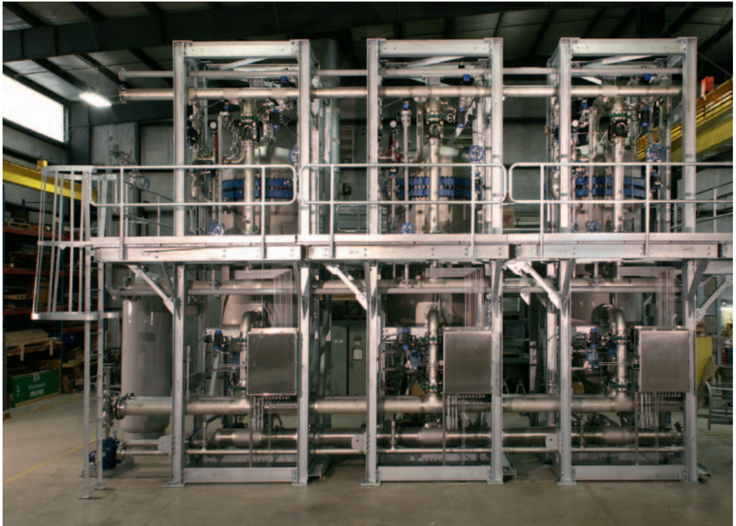
This triplex candle filter system during fabrication are manifolded for concentrated slurry discharge. For this application the system consists of three concentrating candle filters, including piping, wiring to junction boxes. BHS has designed the control system and it is operating by communication with the plant DCS.
