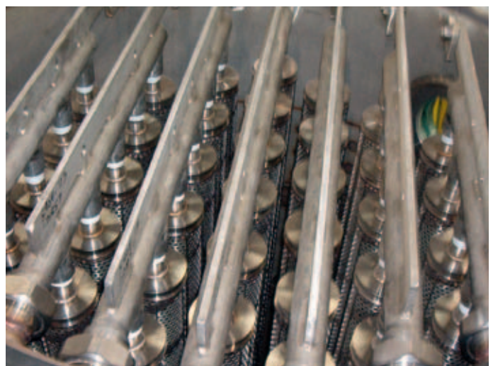
2 BHS candle filter are designed for dry cake discharge and illustrate the candle filter vessel.
