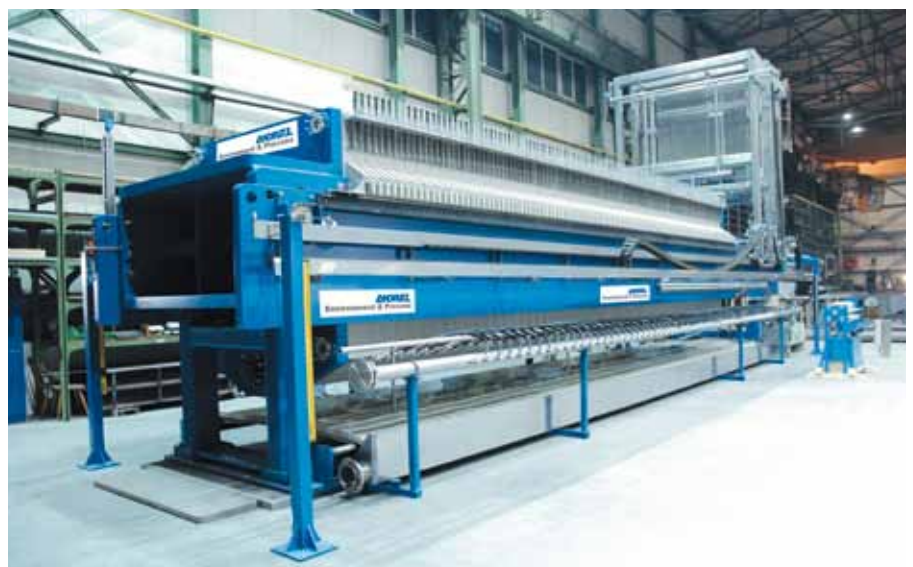
▲ ANDRITZ membrane filter press used to dewater sludge from municipal wastewater treatment plants. The press reduces the sludge volume and produces clear filtrate that can be discharged to the sewer.
