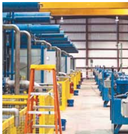
▲ ANDRITZ membrane chamber filter press A4 2000mm x 2000mm with automatic cake discharge
