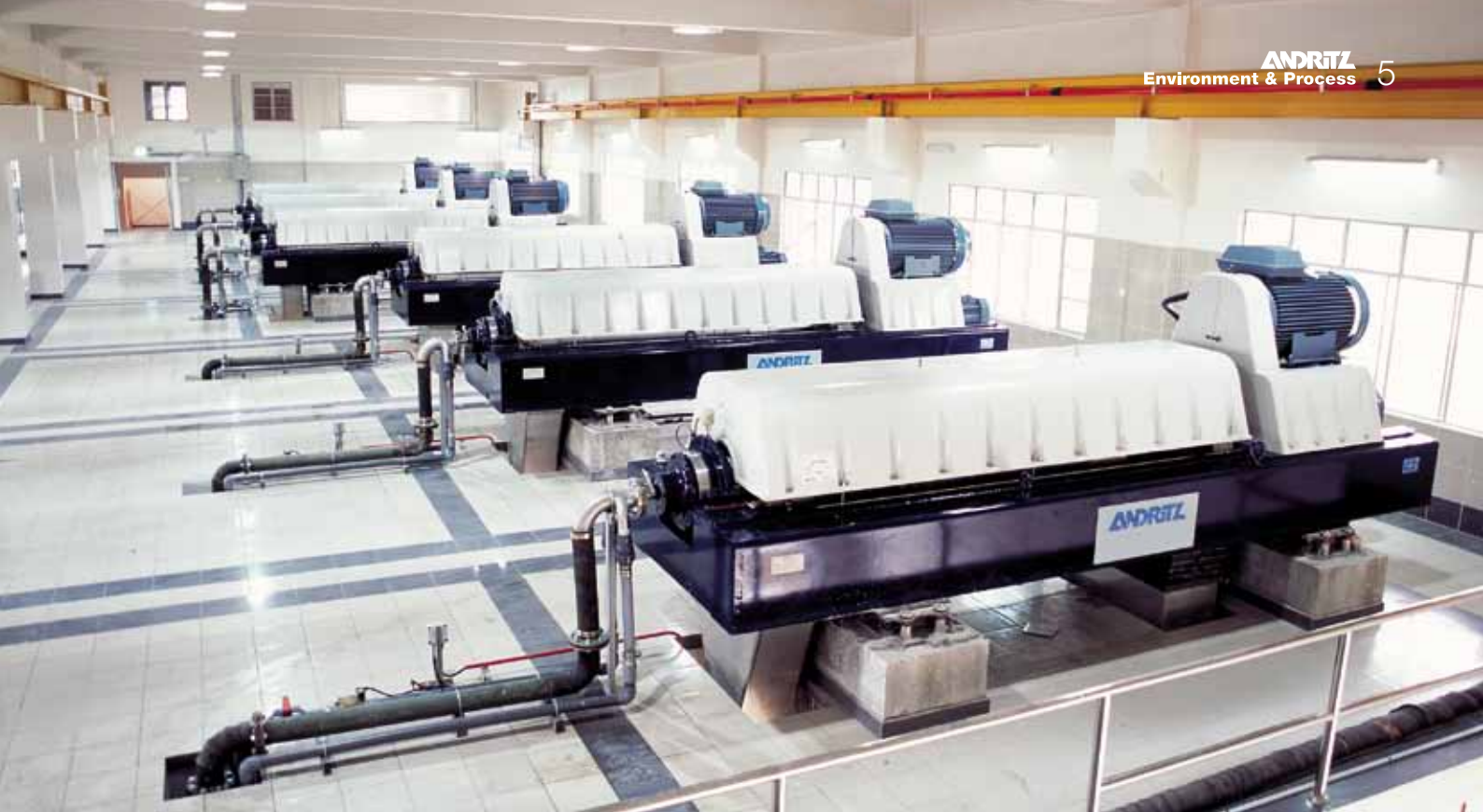
▲ These six D7LL decanters were supplied to Sungai Semenyih, Kuala Lumpur, Malaysia, one of the largest drinking water treatment plants in Southeast Asia. Sungai Semenyih use the decanters to treat the drinking water sludge as a result of the rising ecological awareness of the Malaysian government.
