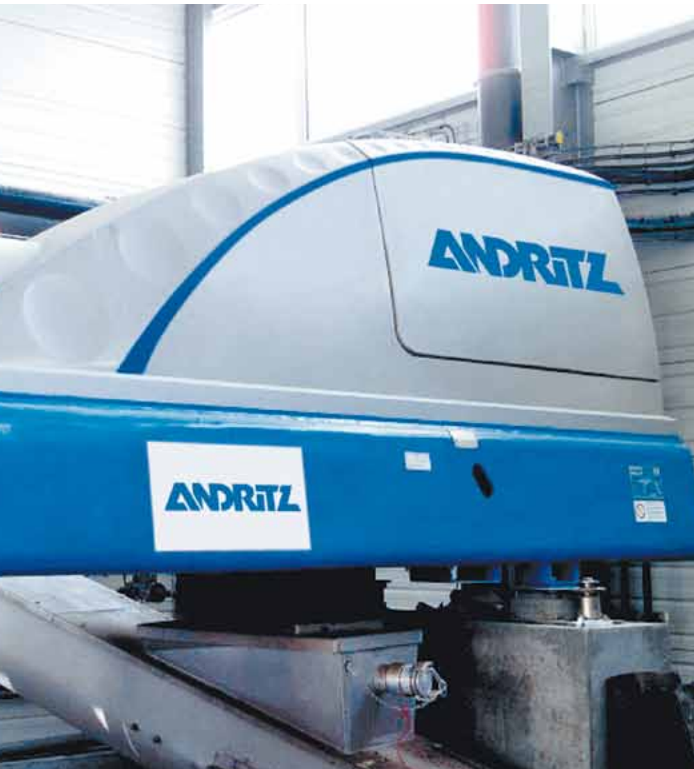
◀ The plant wastewater is digested in a treatment plant equivalent to the size of a 250,000 people town. The sludge from a digestion process (biogas is used to produce power for the plant) is dewatered on an ANDRITZ D4 Series decanter centrifuge to high dryness.
