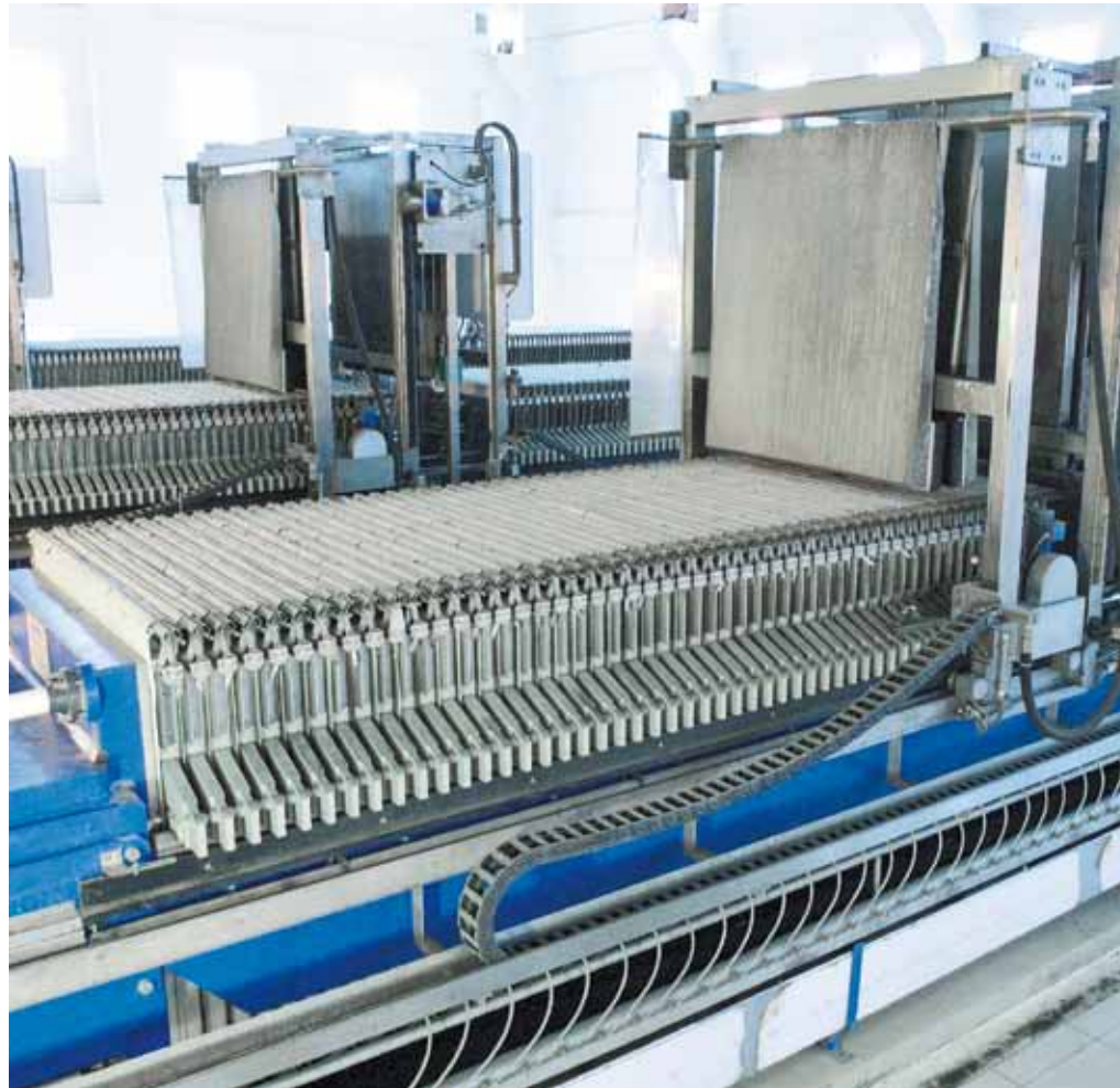
▲ ANDRITZ supplied five fully automatic large-capacity filter presses for water and wastewater treatment in China's largest Industrial Park. Two additional presses have been installed in 2007.
