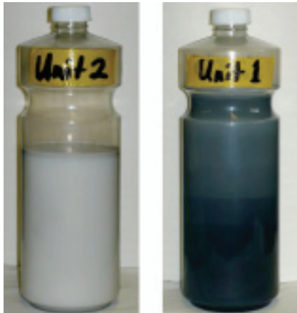
11, 12. Offline soak wash effluent sample for Unit 2 reflects 2505 continuous base-load hours with H12 HEPA filters (left); sample for Unit 1 reflects 1480 base-load hours with conventional filters (right)
