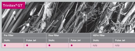
Trinitex® is an Ahlstrom proprietary technology that produces filter media with 3 layers. Layers can be modifed to suit the specific needs of Gas Turbine Air Intake. High strength due to synthetic fibers and Superior performance in diesel soot applications. Trinitex® can be used in both, static and pulse jet applications and well suited for environments with high humidity, soot and salt.
