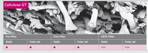
Cellulose GT filter media is a product with blends of polyester and cellulose fibers. Blends are typically 80/20 but can include other ratios as well. Products have good pleatability and excellent performance in dusty environments. Products can be used for pulse jet and static applications.
