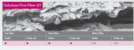
Cellulose Fine-fiber GT filter media is a family of products with a fine layer of Fine Fiber on top of a cellulose carrier sheet. The product offers superior filtration efficiency and dust holding capacity due the very fine layer of small fibers. High corrugation also helps the Pulse Jet cleaning process.
