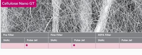
The Cellulose Nano GT filter media products are based on a cellulose carrier media coated with a nano fiber layer based on the electro-spinning technique. Depending on the media combinations a wide range of filtration performance characteristics can be reached.
