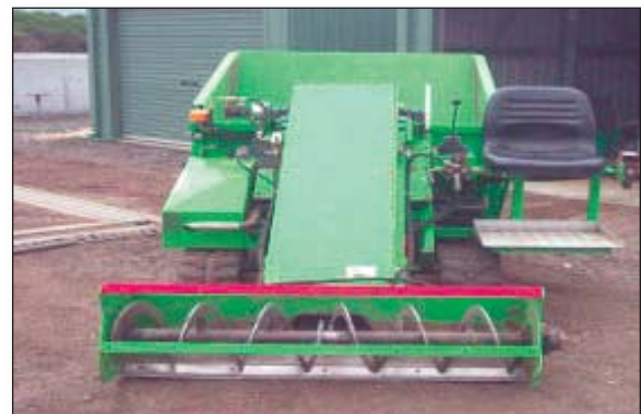
Dried Solids Harvesting Unit
