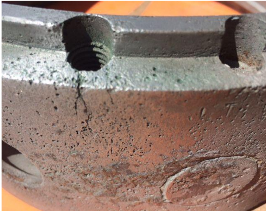
STRESS CORROSION CRACKING
