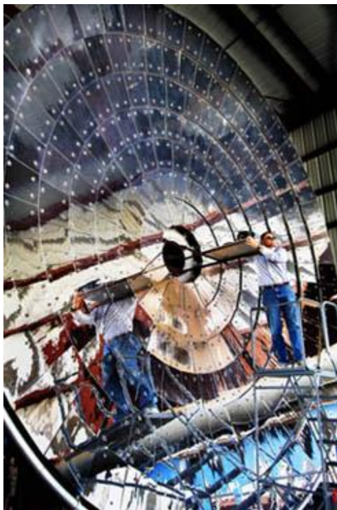
Sandia researcher Rich Diver checks out the solar furnace which will be the initial source of concentrated solar heat for the CR5 prototype. Eventually parabolic dishes will provide the
