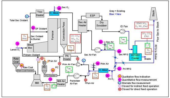
Fig.1 CEDF oxy-combustion equipment and instrumentation.
