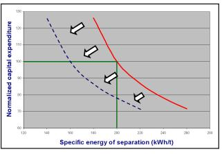
Fig. 10 Tradeoffs of CAPEX and OPEX in ASU design.
