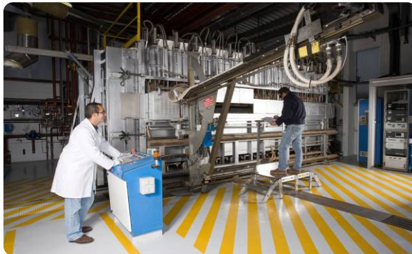
Test combustion platform at Air Liquide R&D center in France
